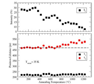
Positron lifetimes  $\tau_1$ ,  $\tau_2$  and intensities  $I_1$ ,  $I_2$  of sample 1 as a function of the annealing temperature.  $\tau_1$  is almost constant and close to the bulk lifetime of as-grown Si.  $\tau_2$  increases from 460 ps after 800 °C to 530 ps after 1227 °C annealing.
