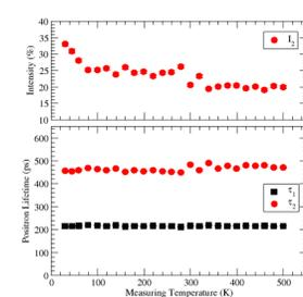
Only two lifetime components can be decomposed. Both lifetime components are independent of the sample temperature.  $\tau_1$  is near to the bulk lifetime (218 ps) of as-grown Si. The lifetime  $\tau_2$  of about 460 ps is related to larger vacancy clusters. The positron lifetime related to dislocation-bound vacancies found after high-temperature deformation has not been observed after RT deformation.
