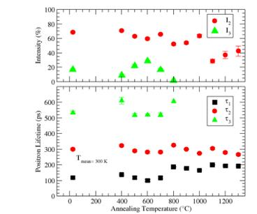
Positron lifetime components  $\tau_1$ ,  $\tau_2$ ,  $\tau_3$  and intensities  $I_1$ ,  $I_2$ ,  $I_3$  of sample 3 as a function of the annealing temperature. All lifetimes are independent of the sample temperature during measurement. The lifetime  $\tau_3$  for vacancy clusters disappeared after annealing at 800 °C.
