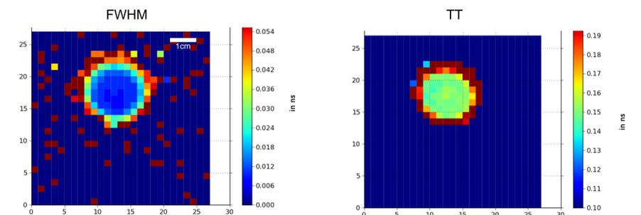
**X-Y scan of the new Hamamatsu H5320:** This is a 10 dynode PMT with a 20mm photocathode and a nominal very short TTS=160 ps (H3370-50: TTS=300ps). The scan shows that the time behavior is very good.
