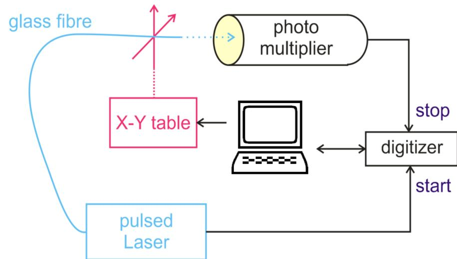
**The setup:** The glass fibre tip scans the photocathode of the PMT. 35 x 35 time spectra are recorded in order to determine the FWHM of the time resolution function and the transition time (TT) locally resolved.
