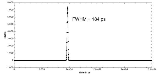
**Single lifetime spectrum of the X-Y scan:** The spectrum was obtained for one spot (2.5x2.5 mm<sup>2</sup>) for the Hamamatsu PMT 3370-50. The resolution and the position on the time axis is recorded for all spots to obtain the X-Y plots across the whole photocathode of the PMT.
