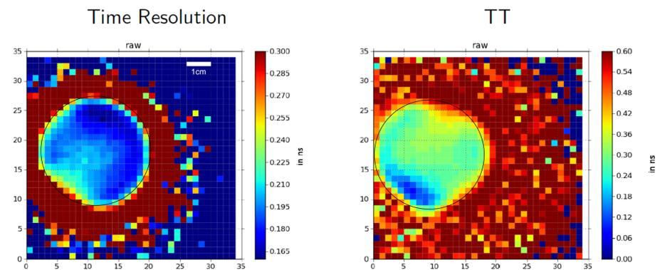
**X-Y-Scans:** The figure shows a scan across a Hamamatsu PMT H3378-50. The locally resolved time resolution (FWHM) and also the transition time (TT) is shown. The photocathode is seen as inner circle of about 45 mm. The outer brownish ring is due to stray light.
