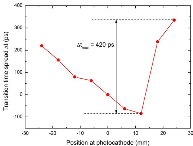
**First experiment:** The first test was performed as one-dimensional scan along the center line of the photocathode of an XP2020Q (not any more in production). The transition time is plotted as function of the position along this line. It is obvious that this particular tube can only be used with a small scintillator of 20 mm diameter, avoiding thus the area at  $r > 10$ mm. In that case TTS  $\approx$  150 ps is acceptable.
