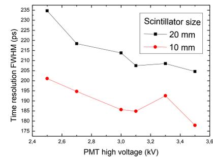
**Time resolution as function of high voltage and scintillator size:** The results of the above X-Y scans were averaged in an area of 10 and 20 mm diameter to see the possible effect of a smaller scintillator size. The high voltage increase will not significantly improve the time resolution when  $U_{HV} > 3.1$  kV.
