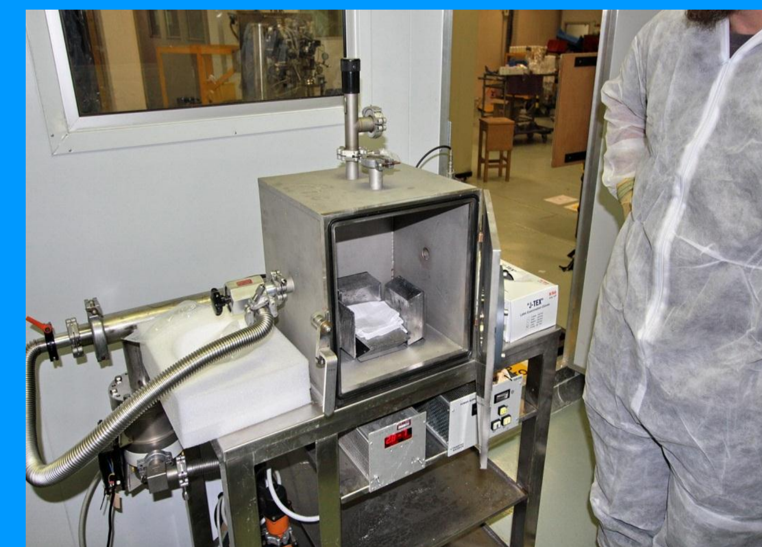
Figure 5. Vacuum Testing of sealed capsules
