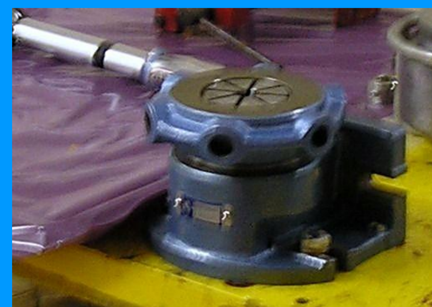
Figure 4. Special holder for sealing of the source.
