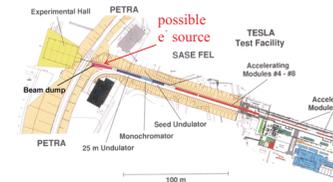
Top view of "TESLA Test Facility - TTF" at DESY in Hamburg. A possible positron beam can be generated in the beam dump area. The experimental setup could be placed to the experimental hall (yellow) or in the small building close to the dump (drawn in black).
