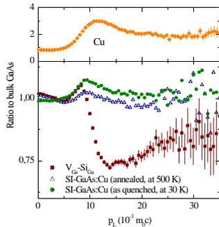
High-momentum part of the positron annihilation momentum distribution, normalized by taking the ratio to a GaAs:Zn reference
