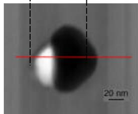
EDX scan and high resolution TEM picture of the large vacancy cluster-Cu-Ga precipitate complex
