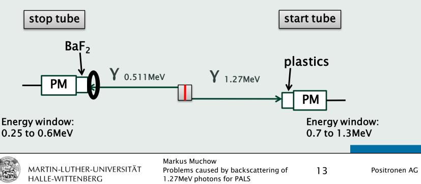
Second idea: start and stop tubes offcentered + Pb-shield with hole in middle in front of stop tube
