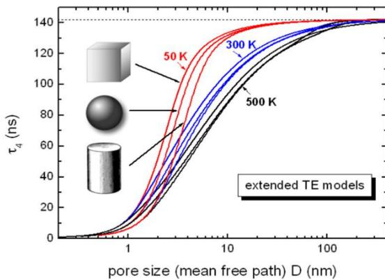
To connect the lifetime with the pore size it is necessary to use a mathematical model for the pore properties. The lifetime depends on temperature and geometry of the pore. A possible relation is described by the extended Tao-Eldrup-Model. Obviously the PALS is very sensitive of differences in pore sizes between 1nm and 30nm.
