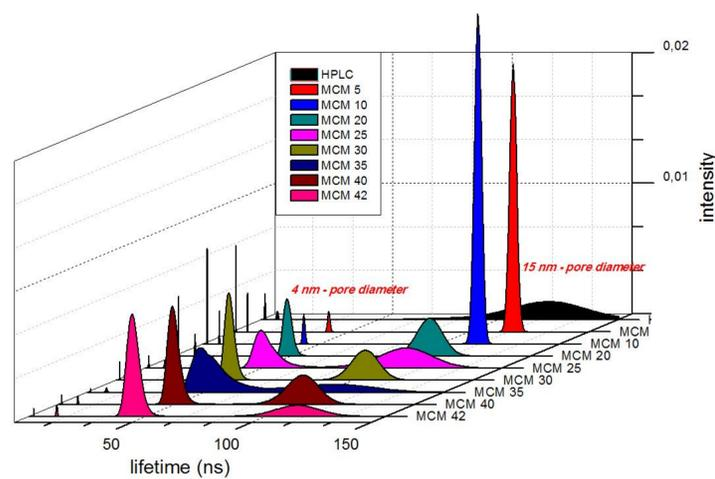
The second example shows an transformation of a porous material. 4nm pores were built into the wall of 15nm pores. The intensity (equal to the number of pores at a discrete lifetime) of the 4nm pores is increasing with the amount of solution.
