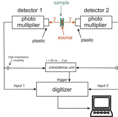
A scheme of the digital PALS is pictured above. To detect the gamma rays photomultiplier (PM) with plastic scintillators are used. Both function as start or stop pulse. The coincidence unit proves whether the signals fit in a set time range and actuates the trigger. The digitizer sends the data to a PC which arranges the pulse to start and stop. To get a full spectra we need to collect at least  $10^6$  events.
